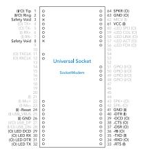
Universal Socket Connectivity. Multi-Tech's universal socket flexible comm-port architecture provides analog dialup, ISDN, wireless, or Ethernet socket connectivity with interchangeable communications devices. This allows you to utilize one system design and populate it with your communications device of choice. In addition, you are assured a seamless migration to future technologies.
